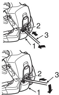
1. Spark plug cover      2. Spark plug cover latch      3. T-wrench
