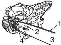
1. Groove      2. Oil hole      3. Guide bar      4. Sprocket
