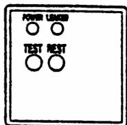
Sensing the earth leakage current, the unit (relay) send a signal To the 3-phase and the 1-phase breaker to trip-off in order to shut-off The circuit to the terminals (loads).
