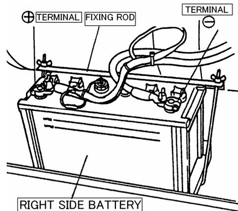
✳️ Reinstall the new battery in the reverse order (always install the cable to the positive (+) post of the new battery first).
