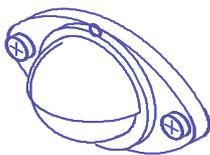
Pilot Lamp indicates whether or not generator is generating electricity, when the engine is driving.
