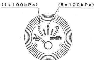
Oil Pressure Gauge displays the pressure of engine oil. Normal pressure may vary depending on the environment, but it should display  $0.98 - 4.9 \times 100\text{kPa}$  ( $1-5\text{kgf/cm}^2$ ). However, under cold weather, the pressure gauge may displays higher reading. Continue idling until the pressure falls to normal range.
