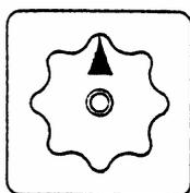
Using this switch, the current between the phases (R.S.T) will be displayed on the Amp meter.
