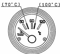
Water Temperature Gauge displays the temperature of engine coolant. Normal temperature may vary depending on the environment, but it should be between 75 to 90 degree Celsius.
