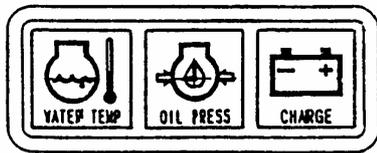
This generator is equipped with monitoring function for water/coolant temperature, oil pressure, battery charge, air filter flow, battery fluid level, and fuel level.
