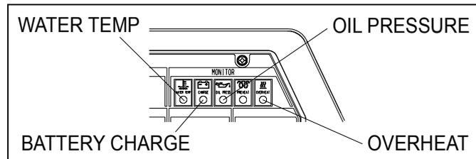
Under normal condition, when the starter switch changes from [STOP] to [RUN], all the lamps of BATTERY CHARGING, OIL PRESSURE and OVERHEAT turn ON. When the engine starts, all the lamps turn OFF. When abnormality is detected on other than OVERHEAT, the corresponding monitor lamp will flash, and the engine automatically shutoff.
